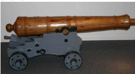
The Barrel 'positive' sitting on the new oak carriage. A new lightweight carriage is to be built for the wooden barrel.
